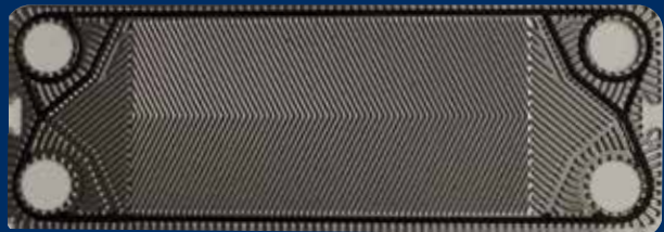
AFTER CLEANING: Varnish film cleaned using VARTECH™ ISC
