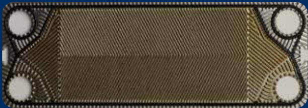
BEFORE CLEANING: Varnish film
